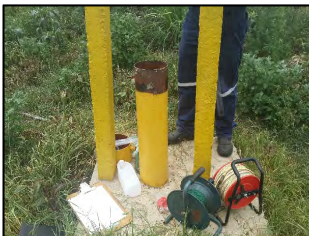
Plate 4: Monitoring and sampling of borehole B 6, located away to the south-east of the proposed site.
