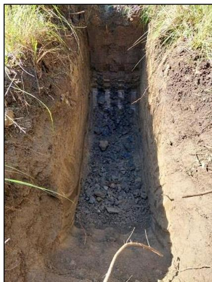
**Plates 11 to 14: Typical soil profiles encountered beneath the site; clayey residual soils overlying the generally shallow, completely to highly weathered shale rock of the Pietermaritzburg Formation. The general dip and dip direction of the shale beds is 10 to 15° to the east.**
