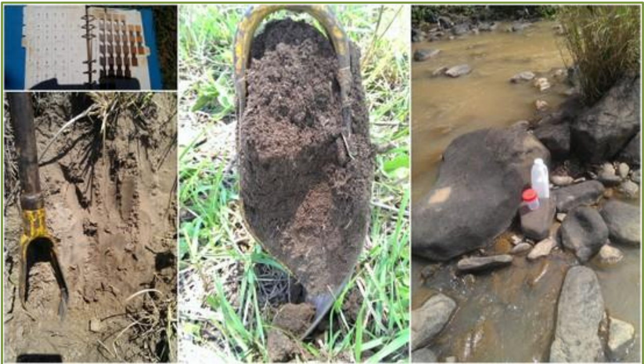
Figure 4 Soil and water quality sampling technique undertaken at Darvill, showing the analysis of soil colour, depth, structure and texture in the dryland area
