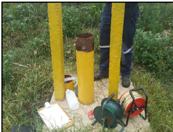
Plate 4: Monitoring and sampling of borehole B 6, located away to the south-east of the proposed site.
